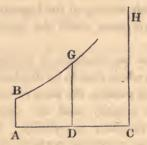
ning of the motion to be represented by the line C A, and after any time by the line C D. The area A B G D will be as the time, and A D as the space described.
